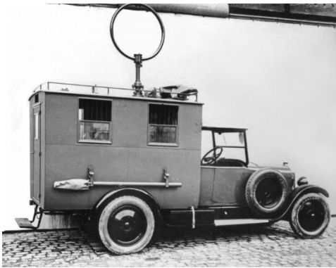
Mobile Peilstation P 29
